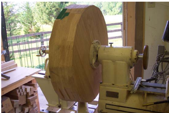
A Greek shield rounded with a chainsaw and then mounted outboard for turning. Before and after.
