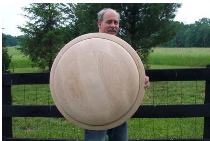
A Greek shield rounded with a chainsaw and then mounted outboard for turning. Before and after.
